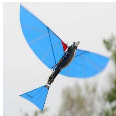
Fig. 1.4.3 IIT Kanpur developed flapping wing MAV
